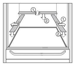
Align the metal strips flush against the side and rear walls of the cabinet
